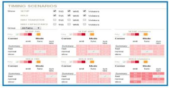
View timing progress with Total Negative Slack, Worst Negative Slack in tabular form, then click on a specific run to view timing corners, and violators for SetUp, Hold, Max. Capacitance, etc. in color coded Timing Corner/-Mode diagrams
